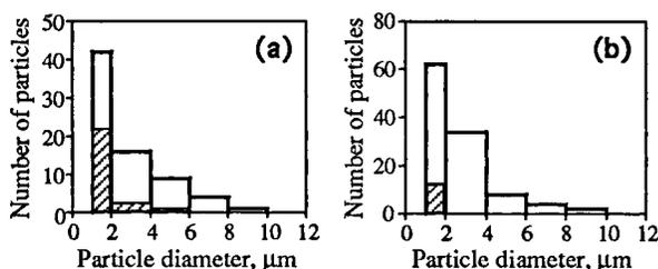
FIG. 5. Distribution of particles by size on a silicon surface on an area 0.018 mm<sup>2</sup> before (light boxes) and after (shaded boxes) 50 laser shots: (a) in ambient air, (b) in vacuum.
