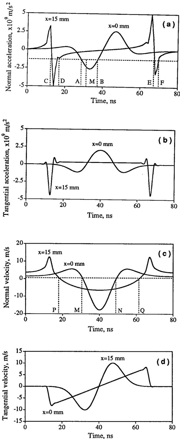
FIG. 2. Surface acceleration and velocity in SAW pulses vs time: (a) normal acceleration, (b) tangential acceleration, (c) normal velocity, and (d) tangential velocity. The waveforms at  $x=0$  mm are calculated using Eqs. (5) and (6), the waveforms at  $x=15$  mm are calculated with the nonlinear evolution Eq. (7) and presented with the time shift equal to the propagation time of a linear SAW.
