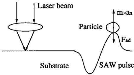
FIG. 1. Schematic diagram of surface cleaning with a laser generated SAW pulse.
