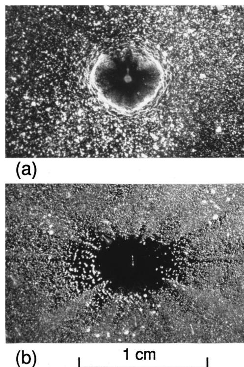
FIG. 3. Photographs of a silicon surface with dust particles after exposure to 50 laser pulses: (a) in ambient air, (b) in vacuum.
