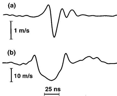
FIG. 4. Measured waveforms for the normal surface velocity component in SAW pulses: (a) excitation in a Si wafer with optical breakdown, quasilinear regime; (b) excitation in fused silica through a strongly absorbing liquid layer, nonlinear regime.
