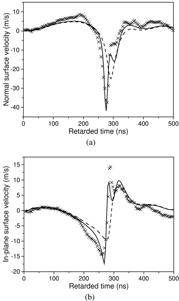
Fig. 2. Calculated waveforms of SAW pulses: (a) normal surface velocity, (b) in-plane surface velocity. Solid lines were calculated with both local and nonlocal nonlinearities taken into account ( $\varepsilon_1 = 0.88$ ,  $\varepsilon_2 = -1.0$ ,  $\varepsilon_3 = 4.0$ ); the dashed lines were obtained with the local nonlinearity only ( $\varepsilon_1 = 0.88$ ,  $\varepsilon_2 = 0$ ,  $\varepsilon_3 = 0$ ). For convenience of comparison experimentally determined waveforms are shown by crosses.
