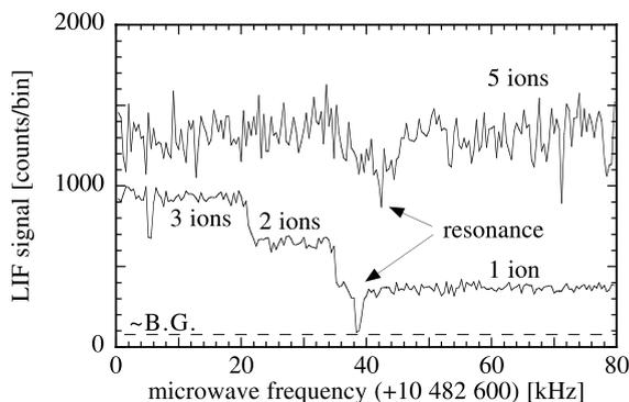
Fig. 7. Test result for crystallized ions made with a few ions (upper trace) and a single ion (lower trace).
