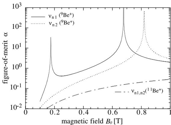
Fig. 2. Figure-of-merit  $\alpha = |g_I/\Delta g_I|/|B_0/\Delta B_0|$  for the nuclear spin flip transitions of  ${}^9\text{Be}^+$  ( $\nu_{n1}$ ,  $\nu_{n2}$ ) and of  ${}^{11}\text{Be}^+$  ( $\nu_{n1,2}$ ) as a function of the magnetic field. The singular points in  ${}^9\text{Be}^+$  mark the *clock* transition conditions. There are no such points for  ${}^{11}\text{Be}^+$ .
