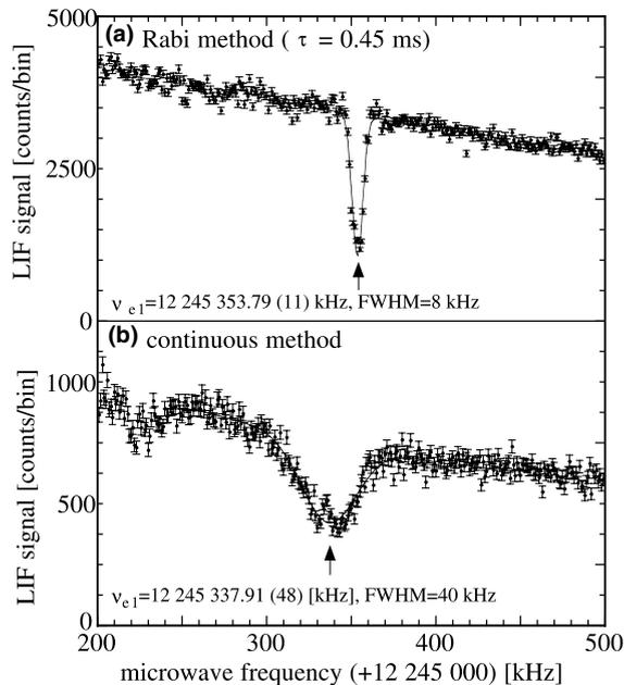
Fig. 4. Microwave resonance spectra for the electron spin flip transition  $\nu_{e1}$  taken by the Rabi method (a) and the continuous method (b). The fluorescence signal was accumulated for a period of 28 pulses per data point (a), and for a continuous period of 500 ms per data point (b).
