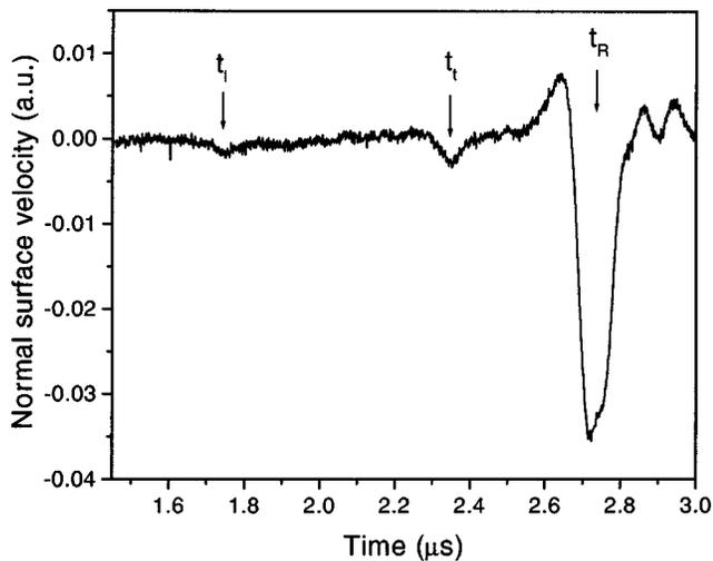
FIG. 3. Surface waves observed on stainless steel. Arrivals of the longitudinal, shear, and Rayleigh waves are indicated by vertical arrows.
