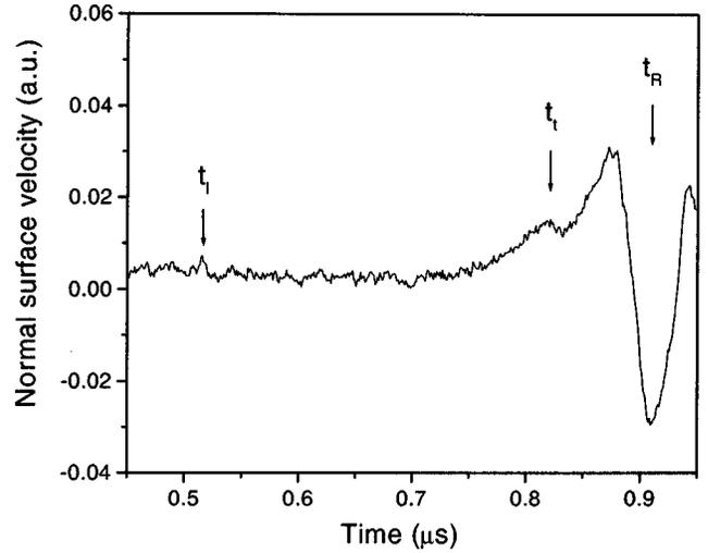
FIG. 1. Surface waves observed on fused silica. Arrivals of the longitudinal, shear, and Rayleigh waves are indicated by vertical arrows.
