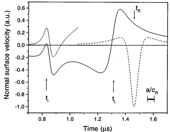
FIG. 2. Normalized wave forms calculated for fused silica. The precursor wave form is shown by a solid line, the Rayleigh wave is presented as a dashed line, and the sum of the initial portion of the Rayleigh wave and the precursor wave form is depicted as a dotted line. The dotted line has the same normalization as the precursor.
