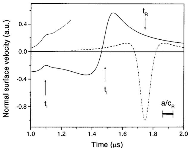
FIG. 4. Normalized wave forms calculated for stainless steel. The precursor wave form is shown by a solid line, the Rayleigh wave is presented as a dashed line, and the sum of the initial portion of the Rayleigh wave and the precursor wave form is depicted as a dotted line. The dotted line has the same normalization as the precursor.
