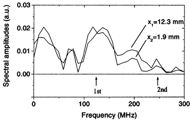
FIG. 5. Spectra of the pulses presented in Fig. 4; first and second harmonics are indicated by arrows.
