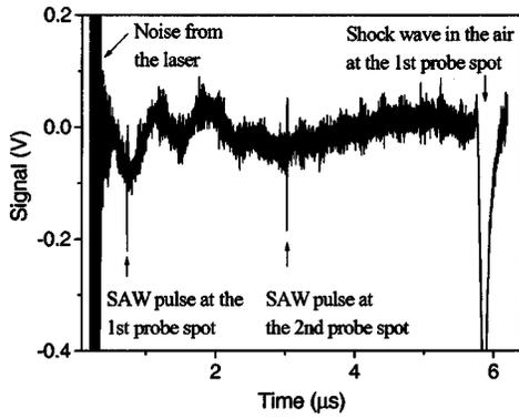
FIG. 2. Signal sequence registered with dual-probe-beam deflection setup.
