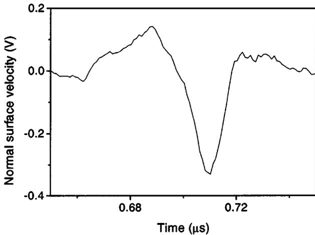
FIG. 3. SAW pulse generated through a liquid layer.
