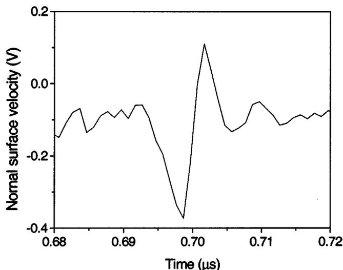
FIG. 1. SAW pulse registered at a free surface of silicon in (001) plane at distance  $x=3.6$  mm from the source.
