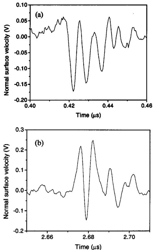
FIG. 4. SAW grating detected at two propagation distances  $x_1=1.9$  mm (a) and  $x_2=12.3$  mm (b).
