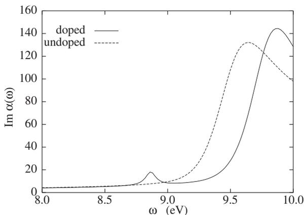
Figure 8. The imaginary part of the frequency-dependent polarizability  $\alpha(\omega)$ . The doped fullerene (solid line) displays a pronounced peak at an energy of 8.8 eV, which compares well with the energy of the transition from the 3s to the 2p state. No such peak is seen in the undoped case (dashed lines). For clarity, we do not show other transition peaks which are similar and common to both the doped and undoped case.
