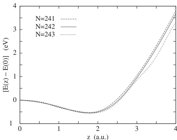
Figure 2. The energy difference between the displaced and centred  $\text{Mg}^{++}$  ion as a function of the off-centre displacement  $z$ , for singly positive ( $N=241$ ), neutral ( $N=242$ ) and singly negative charged ( $N=243$ ) endohedral systems. The energy minimum is about 0.6 eV below the on-centre energy at  $z=0$ .
