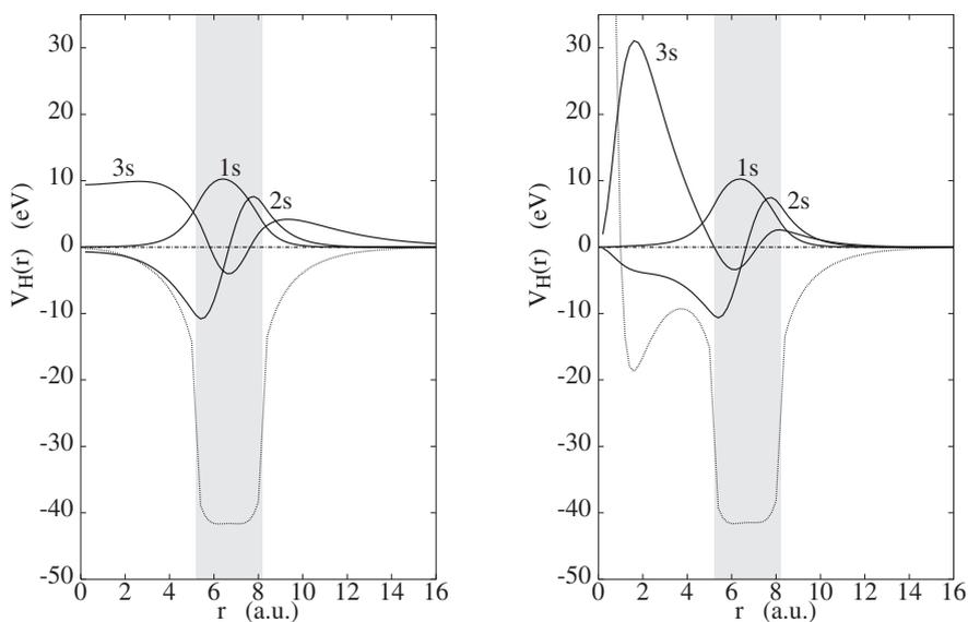
Figure 6. The 1s, 2s and 3s wave function for an undoped fullerene (left figure, solid lines, arbitrary scale) and for a fullerene doped with a  $Mg^{++}$  impurity at the centre (right figure, solid lines, arbitrary scale). Also shown for comparison is the self-consistent potential  $V_H(r)$  (dashed lines, left scale). The grey-shaded areas indicates the range of the jellium background.
