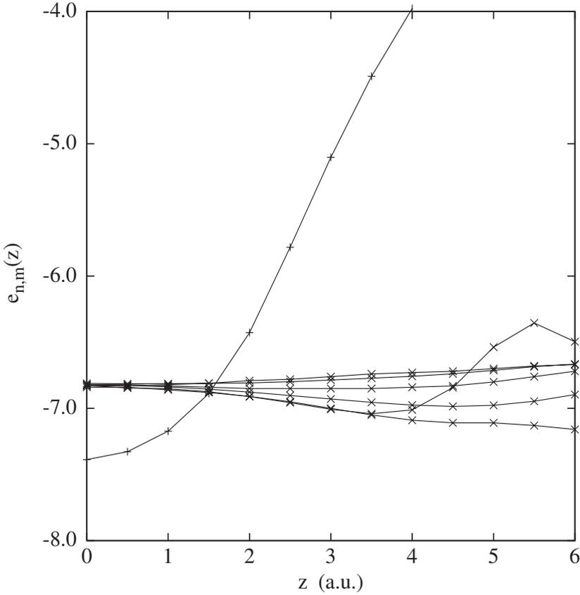
Figure 7. The change in the energy of the 3s state (solid line with + markers) as well as the  $\ell = 5$  states (dashed lines with  $\times$  markers) as a function of the displacement  $z$  of the  $\text{Mg}^{++}$  ion from the centre of the fullerene cage. The lifting of degeneracy as the ion moves off-centre is clearly visible.
