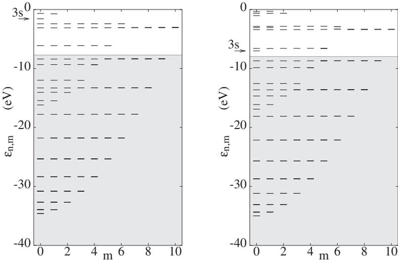
Figure 5. The bound state single-particle spectrum  $\epsilon_{n,m}$  for an undoped fullerene (left figure) and for a fullerene doped with a  $Mg^{++}$  impurity at the centre (right figure). Note the degeneracy of the states for different azimuthal quantum number  $m$ . Note also the shift of the 3s state (pointed to by arrows) between the doped and the undoped case. The grey-shaded area identifies the occupied states.
