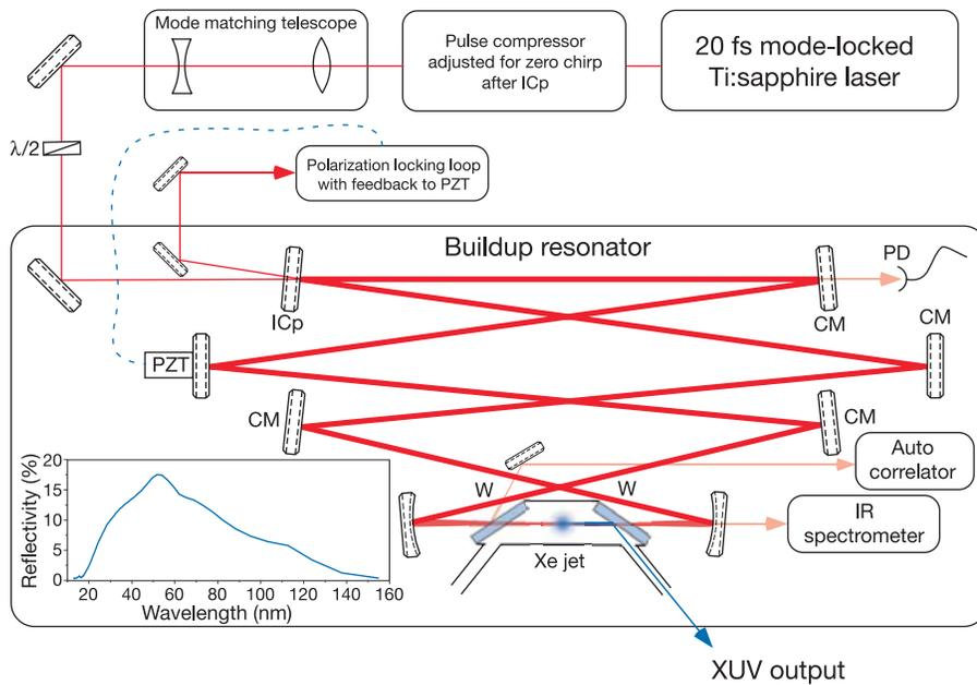
**Figure 1 | The XUV laser set-up.** IC<sub>p</sub>, coupling mirror with 1% transmission; CM, chirped mirrors; PD, photodiode; W, Brewster-angled sapphire window of 1 mm thickness; PZT, piezoelectric transducer. Inset shows the reflectance of sapphire for p-polarized XUV light at an incidence angle of 60.4° (Brewster angle for 800 nm radiation).
