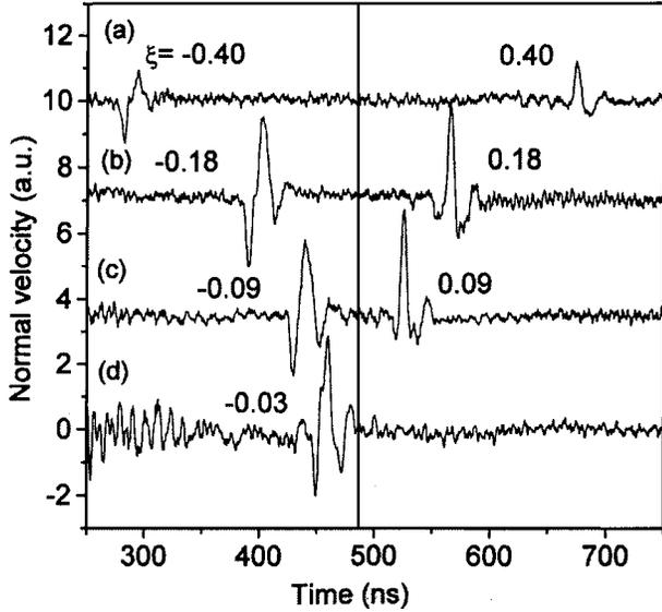
Fig. 1. Pulse shapes observed at several relative distances  $\xi = (x - R_0)/R_0$  from the focus. Pulses (a)–(c) were detected with the excitation in a full circle. Pulse (d) was registered with the excitation in a semicircle,  $x < R_0$ .
