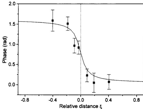
Fig. 3. Dependence of the average phase of the spectral components on relative distance  $\xi$  from the focus. Experimental data are shown by filled squares; the calculated dependence is shown by the solid curve. The vertical dotted line indicates the position of the focus.
