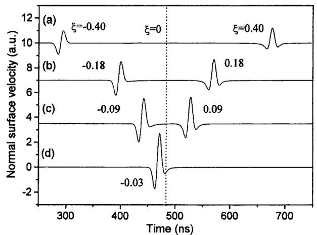
Fig. 2. SAW pulses calculated with the inverse Fourier transform of  $\tilde{v}(\omega)$  from Eqs. (4) for the same relative distances as in Fig. 1. The dotted line shows the arrival time for  $\xi=0$
