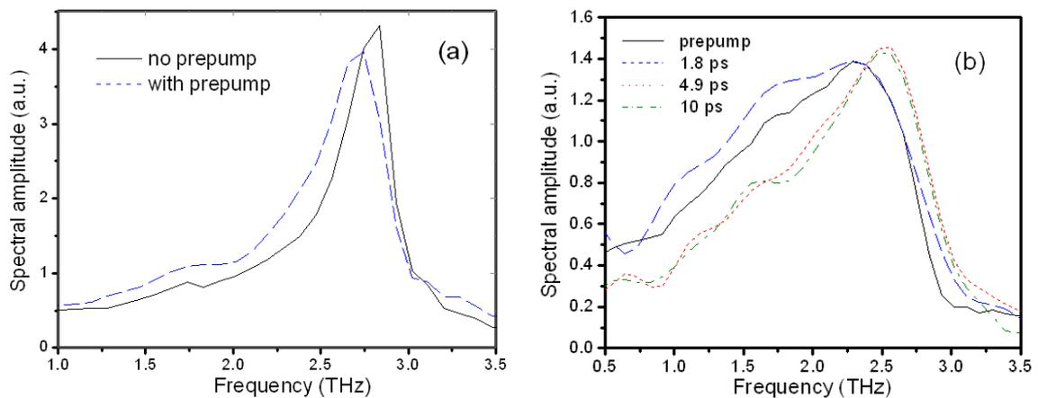
**Figure 5.** Spectra of the oscillating traces, corresponding to the pump pulse: (a) For signals shown in Fig. 4(a) (laser flux  $3 \text{ mJ/cm}^2$ ). (b) For laser flux of the pre-pump  $12 \text{ mJ/cm}^2$ . In case (b) strong frequency shift and spectral broadening are observed for small time delays; relaxation and carrier diffusion lead to narrowing of the spectrum and an increase of the optical phonon frequency for longer delays.
