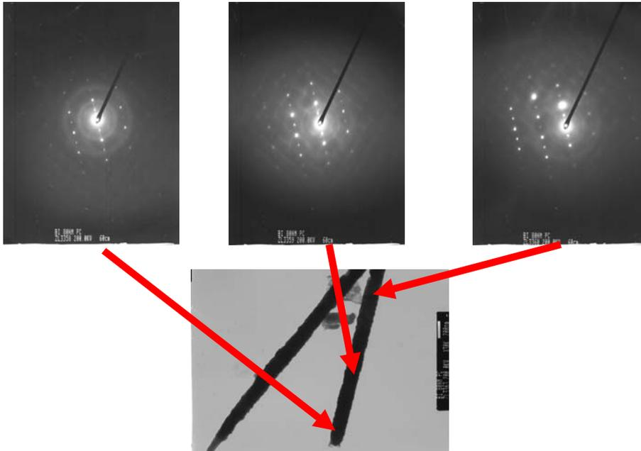
**Figure 1.** The similarity of the TEM diffraction patterns (top figures) registered from different parts of a Bi nanowire (bottom figure) confirms that it consists of relatively large crystallites.
