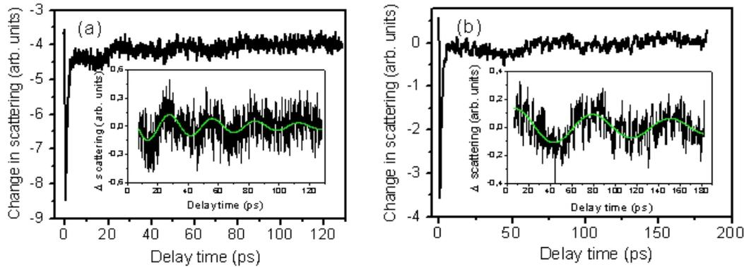
**Figure 3.** Transient signals measured (a) with thin ( $d \approx 63$  nm) Ag nanowires and (b) with thick ( $d \approx 200$  nm) Ag nanowires. Insets show the oscillating parts of the signals fitted by a damped cosine function.
