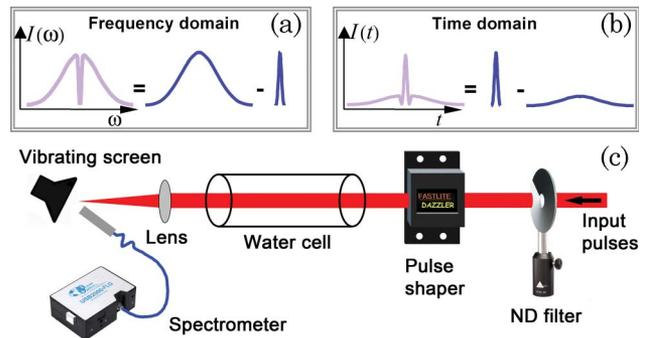
Fig. 1. (Color online) Spectral-hole-filling experiment: (a) Frequency domain and (b) time domain schematics. (c) Experimental setup (femtosecond laser oscillator not shown). Initial 7 fs laser pulses pass through the pulse shaper, which produces a spectral hole and reduces the total spectral bandwidth, and enter the water cell. The transmitted spectra are measured by the spectrometer.
