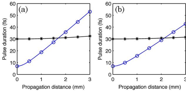
Fig. 7. (Color online) Calculated pulse duration versus propagation distance (a) in K7 glass and (b) in water for two transform-limited input pulses of 7 fs (blue lines and circles) and 30 fs (black lines and stars) initial duration (both at an 800 nm center wavelength). In both figures, the data points show the results calculated with the actual wavelength-dependent refractive indices, while the lines are obtained with the group velocity dispersion (GVD) approximation.
