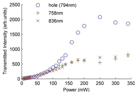
Fig. 5. (Color online) Transmitted intensity for three wavelengths as a function of input laser power. The three wavelengths correspond to the low-power spectral hole center (794 nm) and two wavelengths at the spectral wings (758 and 836 nm) having, at low input powers, the same spectral intensity as the hole center.
