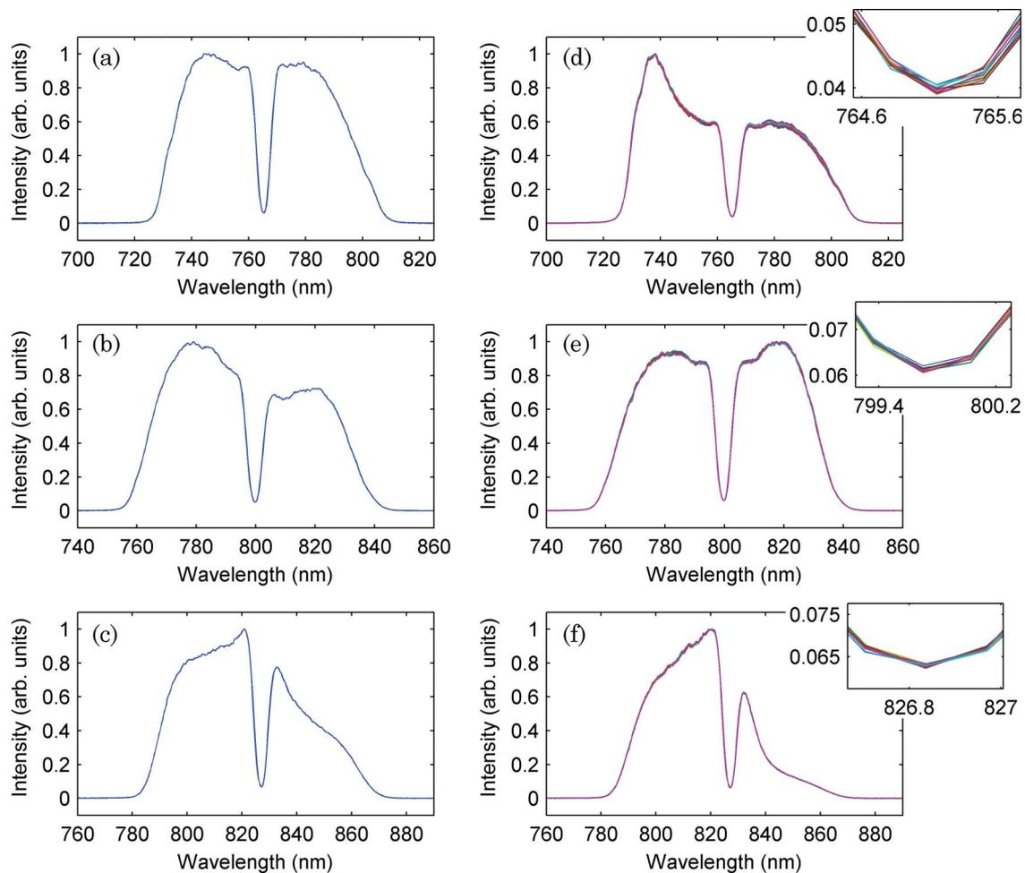
Fig. 2. (Color online) Results from the spectral hole filling experiment with low-power (laser oscillator) shaped pulses. Parts (a)–(c) show input spectra with the spectral hole centered at (a) 767 nm, (b) 800 nm, and (c) 827 nm wavelengths. Parts (d)–(f) show the corresponding output spectra after propagation through 1.15 m of distilled water; insets show zoomed-in spectral hole regions.
