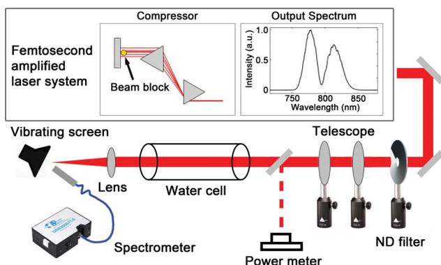
Fig. 3. (Color online) Experimental setup for measuring propagation of amplified laser pulses through water. An obstruction is placed in the compressor to produce a hole in the laser spectrum. Then the pulses propagate through the water cell, and the transmitted spectra are measured by the spectrometer.
