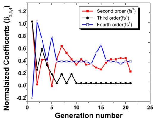
Fig. 7. (Color online) Typical convergence of the second-, third-, and fourth-order dispersion coefficients for TPF optimization.
