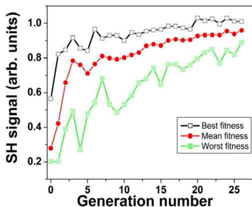
Fig. 4. (Color online) Convergence curves for optimization of the SHG signal. Three different curves show the best, worst, and mean SHG values.
