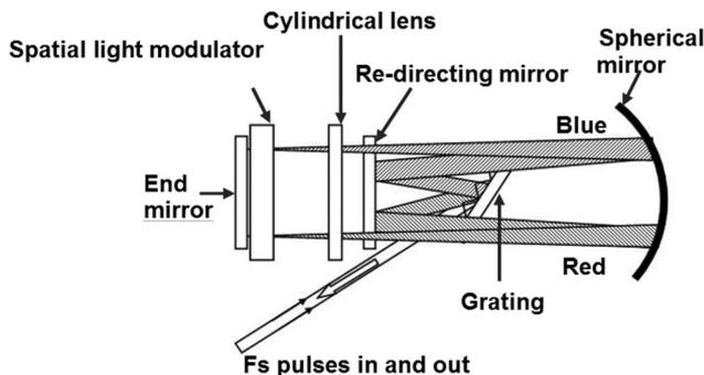
Fig. 2. Schematic diagram of folded 4f setup (top view).
