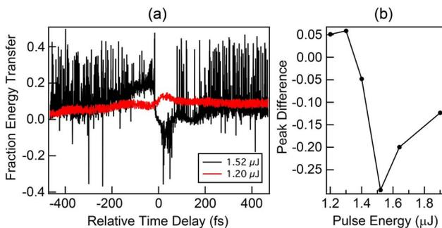
Fig. 2. (Color online) (a) Fraction of energy transfer versus pulse delay for input energies of  $1.20 \mu\text{J}$  and  $1.52 \mu\text{J}$ . (b) Difference between fraction of energy transfer curve extrema for several pulse energies.
