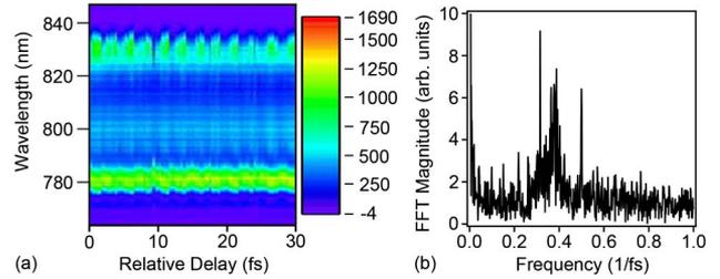
Fig. 3. (Color online) (a) Typical raw spectral measurement of a filament involved in energy transfer in liquid methanol as a function of relative pulse delay. Such raw measurements are spectrally integrated to yield energy transfer curves of Fig. 2(a). (b) Typical FFT of an energy transfer curve for filament-forming, intersecting laser pulses. This FFT peak was completely absent for intersecting pulses that did not form filaments.
