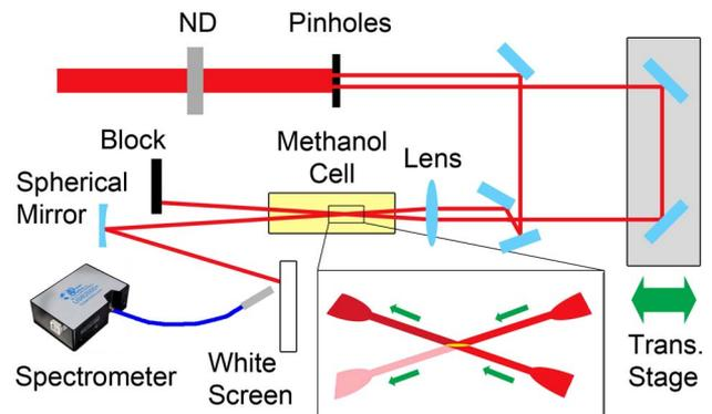
Fig. 1. (Color online) Experimental schematic filter: ND, neutral density. The inset shows the intersection of two filaments involved in energy transfer.
