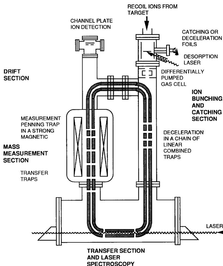
Fig. 7. Proposed linear combined trap for the HRIBF-facility.
