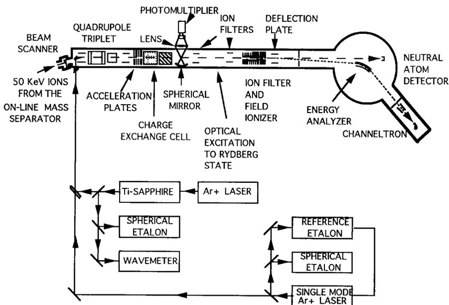
Fig. 6. Experimental apparatus for collinear fast beam laser spectroscopy using two step excitation and field ionization with charged particle detection.
