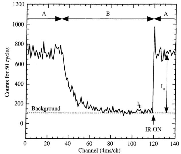
Fig. 2. Fluorescence intensity as a function of time showing the present method in the case of a weak UV laser ( $1\mu\text{W}$ ). The fluorescence spike at the moment when the IR lasers are turned on indicates the number of ions in the trap (For details, see text.)
