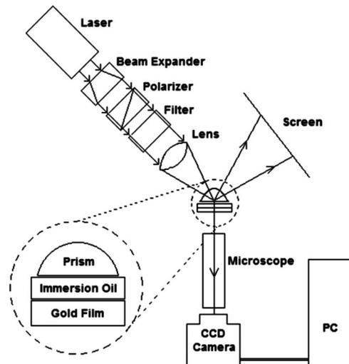
Fig. 1. Experimental setup for studies of surface plasmons.
