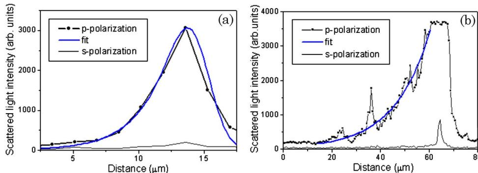
Fig. 4. (Color online) Measured distribution of the scattered light intensity near the laser illumination stripe for (a) 633 nm and (b) 805 nm.
