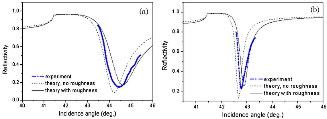
Fig. 2. (Color online) Measured and calculated SPR curves for (a) 633 nm and (b) 805 nm.
