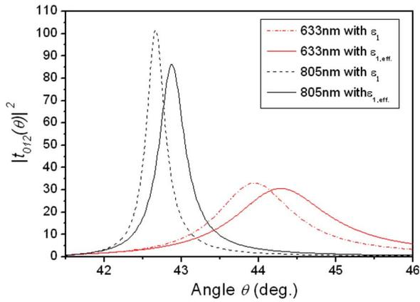
Fig. 5. (Color online) Dependence of the factor  $|t_{012}(\theta)|^2$  on the angle for two wavelengths 633 and 805 nm, calculated for  $\epsilon_1$  from [30] and the corresponding effective dielectric constant of the gold film,  $\epsilon_{1,eff}$ .
