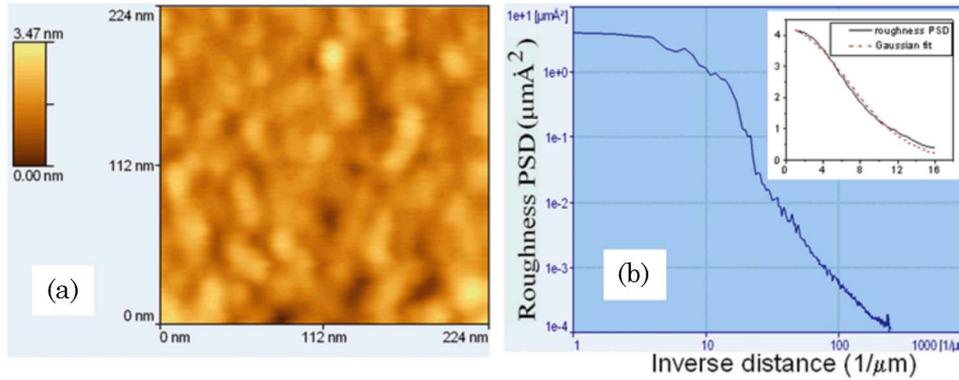
Fig. 3. (Color online) Surface roughness measured with AFM: (a) false color surface relief and (b) the PSD function of the surface roughness in logarithmic scale. The inset shows the fitting of the PSD function by  $\tilde{G}_1(k)$  of Eq. (12) with  $\delta = 2.0$  nm and  $\sigma = 36$  nm [axes have the same units as in Fig. 3(b)].
