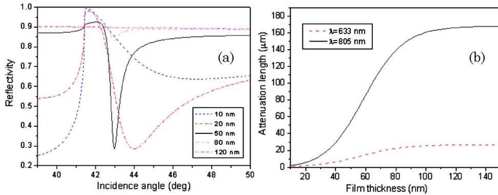
Fig. 7. (Color online) Influence of the thickness of the gold film on the properties of SPs: (a) SP resonance curves at 633 nm for different film thicknesses, (b) the dependence of the attenuation length on the film thickness for 633 and 805 nm. The dielectric constants from [30] are used.
