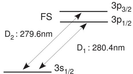
FIG. 1: The  $\text{Mg}^+$  resonance doublet near 280 nm is isoelectronic to the 3s-3p doublet in Na historically labeled as  $D_1$  and  $D_2$  Fraunhofer lines. From the  $D_1$  and  $D_2$  transition frequencies measured in  $^{24}\text{Mg}^+$  and  $^{26}\text{Mg}^+$  we deduce isotope shifts and fine structure splittings (FS). The measurement accuracy allowed to resolve the isotope shift of the fine structure splitting for the first time.
