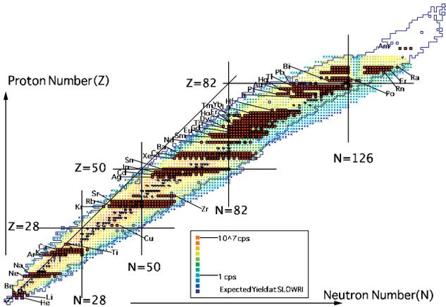
**FIGURE 1.** Expected nuclides at SLOWRI. The dark boxes indicate nuclei which have been studied with optical spectroscopy [2]
