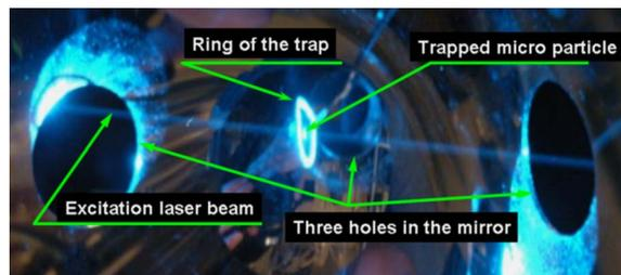
FIG. 2. (Color online) A view of the trap with stored DPA particle that were placed inside an elliptical mirror for measurements of Raman scattering.
