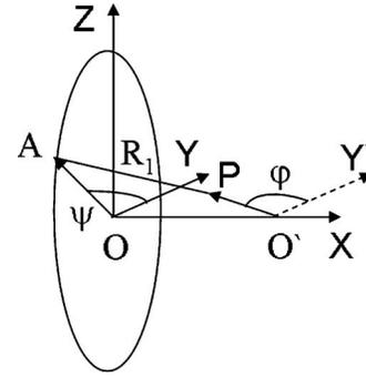
FIG. 9. The geometry of the problem for calculation of electric forces:  $O$  is the center of the ring trap,  $P\{x, y, z\}$  is the position of the particle,  $O'Y'$  is parallel to the axis  $OY$ ,  $OO'=x$ ,  $OA=r_1$ , and  $OP=r$ . The integration is performed over all points  $A$  on the ring.
