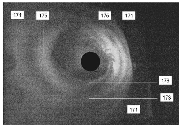
FIG. 7. The diffraction pattern of the backscattered light from a  $9.6\ \mu\text{m}$  particle. The numbers show the calculated angular positions (in degrees) of the bright circles in the backscattering relative to the incident beam.
