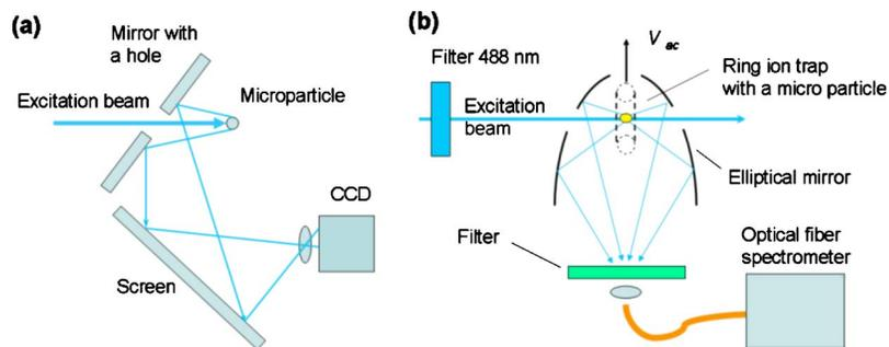
FIG. 1. (Color online) Experimental arrangements: (a) For observation of scattering diffraction patterns from microparticles and (b) for measurement of Raman scattering with an elliptical mirror and an optical fiber spectrometer.
