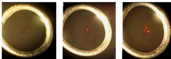
FIG. 6. (Color online) Storage of particles in a ring-type trap: One, two, and several particles. These dipicolinic acid particles are about  $30\text{--}50\ \mu\text{m}$  in size. For observation, they were illuminated by a He-Ne laser beam.
