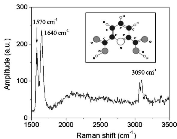
FIG. 8. Raman spectrum corrected for the filter transmission of a single DPA microparticle stored in the electrodynamic trap. The insert shows the structure of the DPA molecule.
