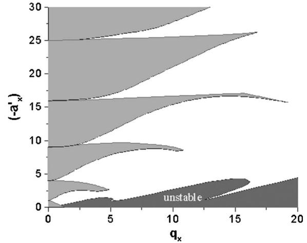
FIG. 3. The diagram shows several regions of highest stability (adjacent to the  $-a'_x$  axis) and an unstable region (the area adjacent to the  $q_x$  axis).
