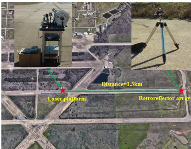
Fig. 2. The aerial view of the 1.3 km measurement path at the TAMU RELLIS Campus along one of the aircraft runways. The laser platform (shown in the left inset) was on a movable cart, the retroreflector (the right inset) was mounted on a tripod standing at the end of the runway.
